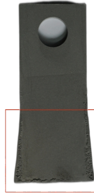
▶ With tungsten carbide and after sandblasting
