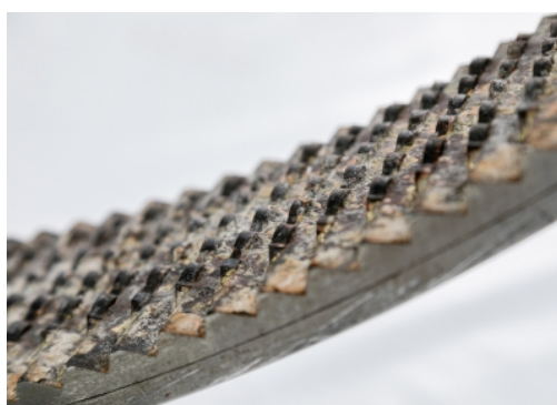
Ring Gear with welded alloy
